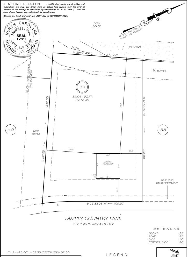
THIS PROPERTY IS NOT LOCATED IN THE 100 YEAR FLOOD ZONE. EXISTING IRON PIPE IRON PIPE SET RIGHT OF WAY NOW OR FORMERLY FES FLARED END SECTION
