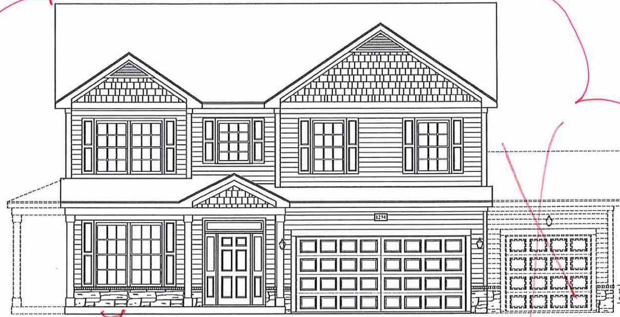
FRONT ELEVATION-A-2 SCALE: 1/4" = 1'-0"
