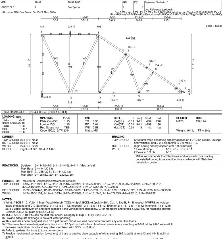
8) This truss is designed in accordance with the 2015 International Building Code section 2306.1 and referenced standard ANSI/TPI 1.
