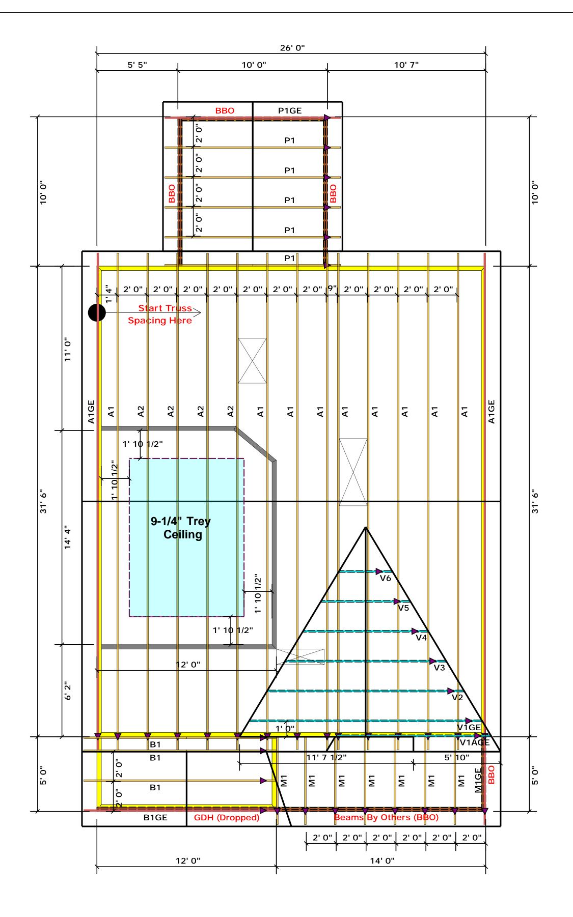
▲ = Denotes Left End of Truss (Reference Engineered Truss Drawing)
