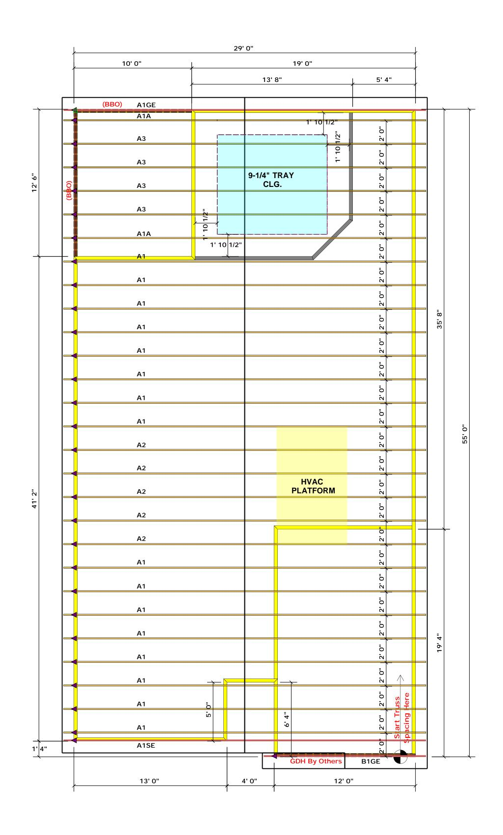
Truss Placement Plan SCALE: 1/4" = 1'-0"
