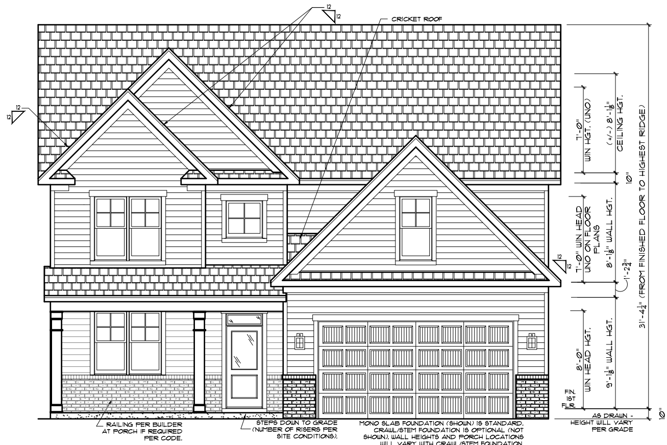
FRONT ELEVATION - CLASSIC 22x34 PRINTS SCALE: 1/4"=1'-0" 11x17 PRINTS SCALE: 1/8"=1'-0"
