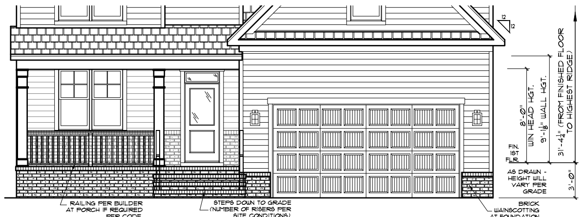
FRONT ELEVATION w/ CRAWL FND. 22x34 PRINTS SCALE: 1/4"=1'-0" 11x17 PRINTS SCALE: 1/8"=1'-0"
