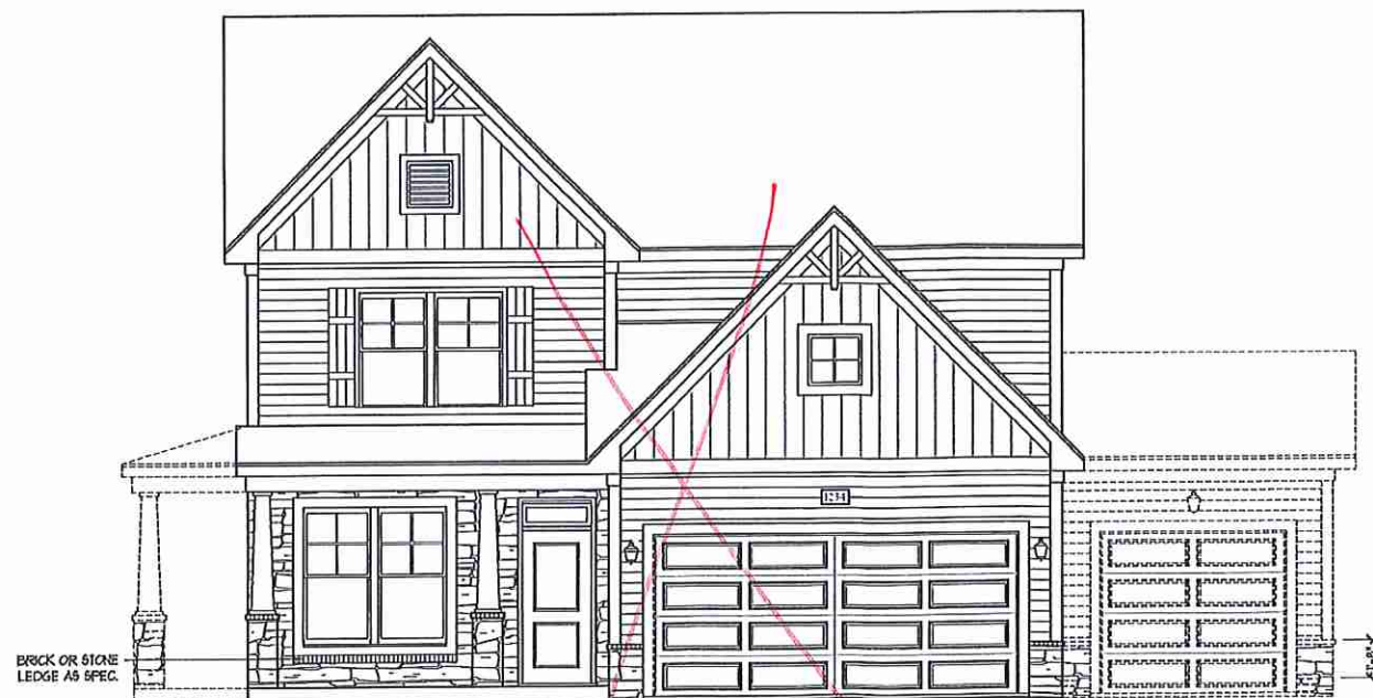
FRONT ELEVATION-B-3 (W/ STONE) SCALE: 1/4" = 1'-0"
