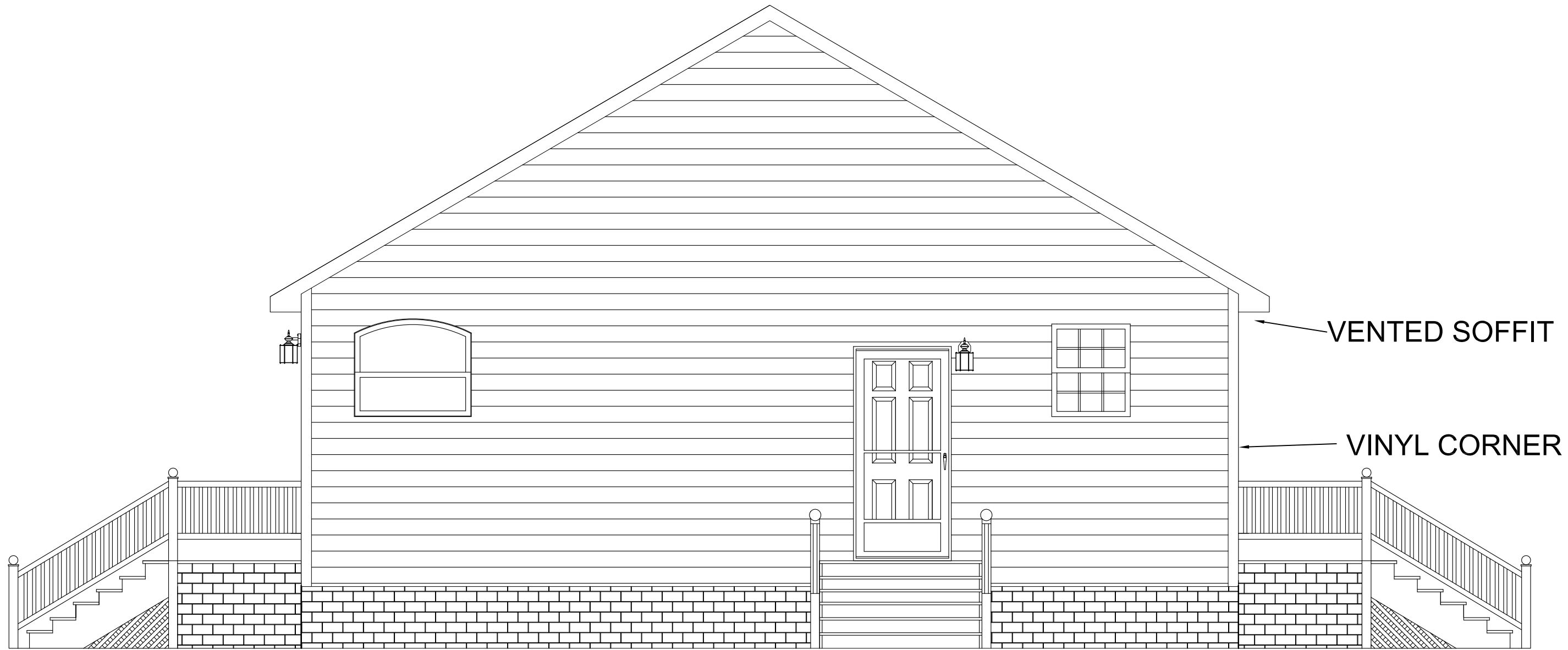
RIGHT ELEVATION FOUNDATIONS, STEPS, PORCHES AND RAILS DONE ON SITE BY OTHERS
