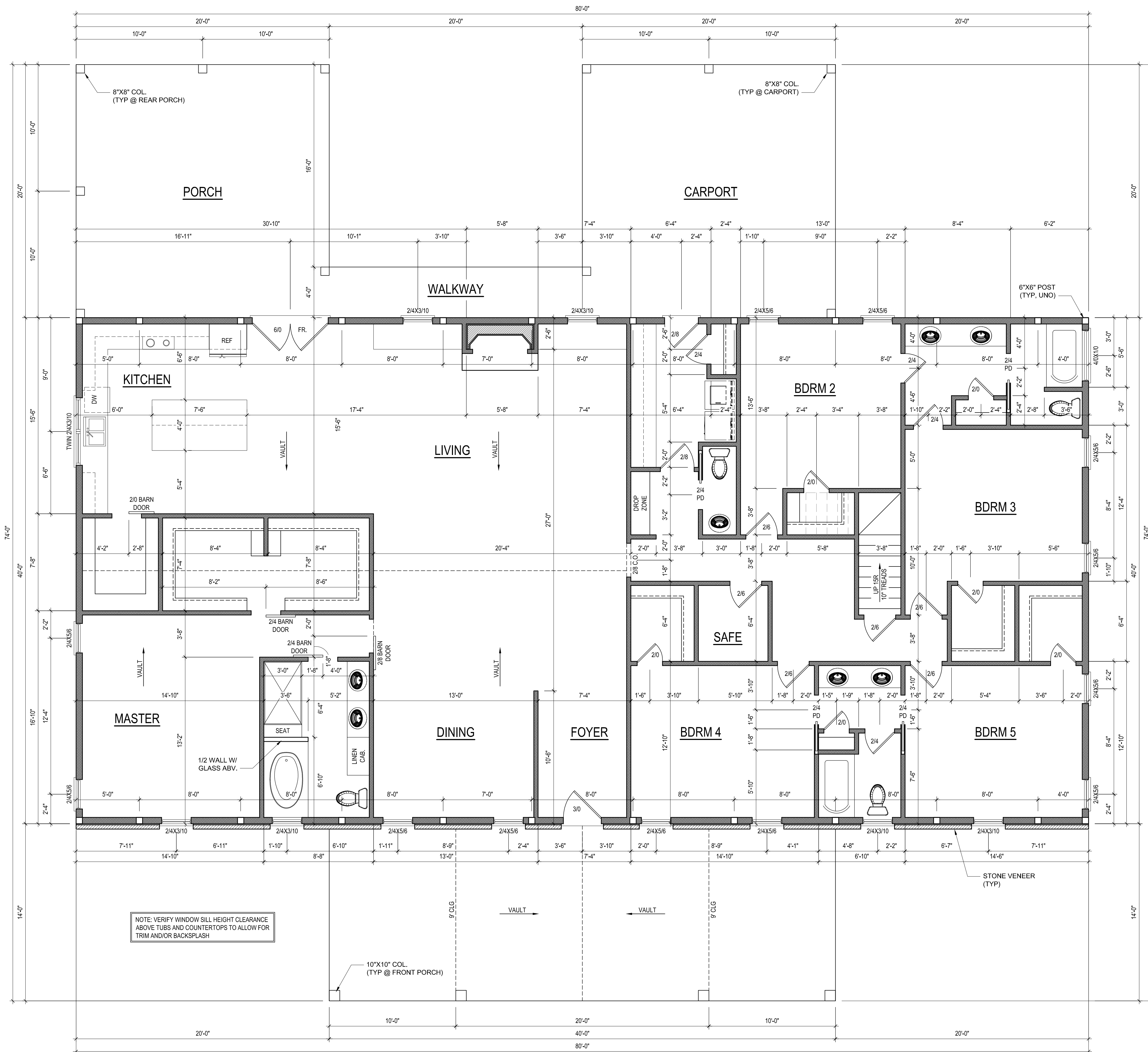
FIRST FLOOR PLAN 1/4" = 1'-0" CLG HGT. = 9'-0" (UNO)
