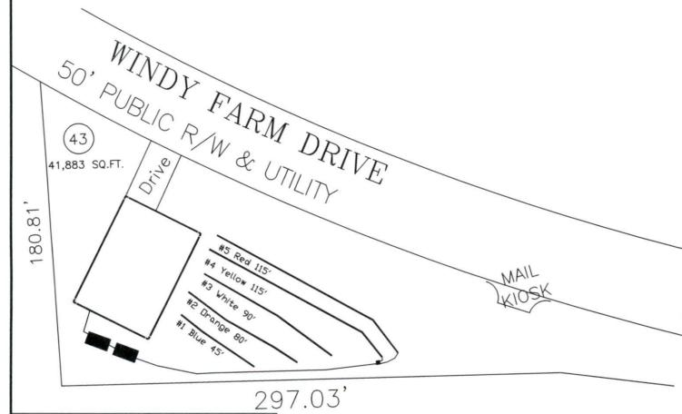
System: Pump to D-Box Lines: 4-5 (230') 0.4 LTAR 24' Trench Bottom Accepted Status System Repair: Pressure Manfiold Lines: 1-3 (215') 0.4 LTAR 24 Trench Bottom T&J Panel System - 50% Reduction
