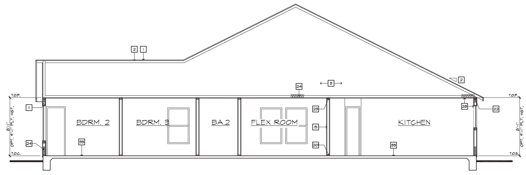
SECTION "B" SCALE 1/4"=1'-0" (22"X34") - 1/8"=1'-0" (11"X17") AT SLAB-ON-GRADE
