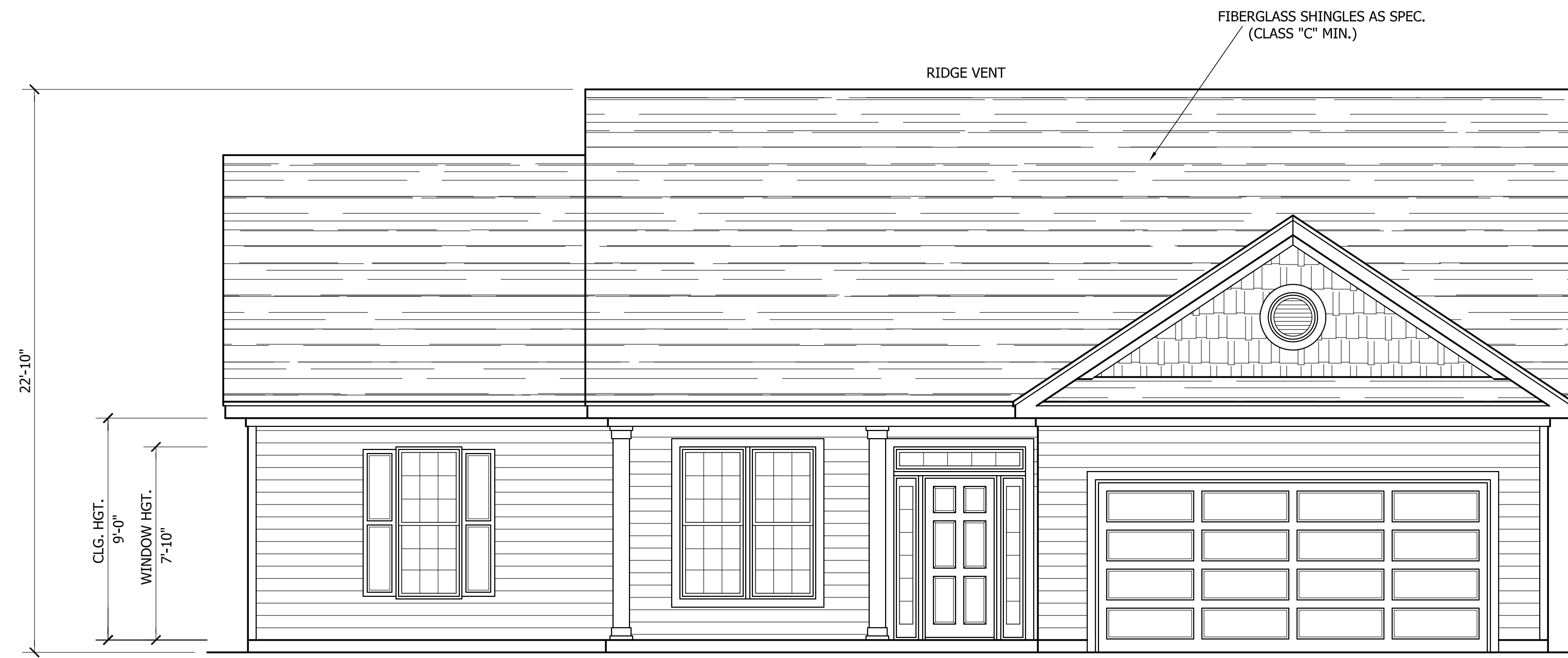
FRONT ELEVATION SCALE: 1/4"=1'-0"
