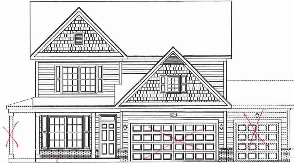
Brick FRONT ELEVATION-A-2 (W/ BRICK) SCALE: 1/4" = 1'-0"
