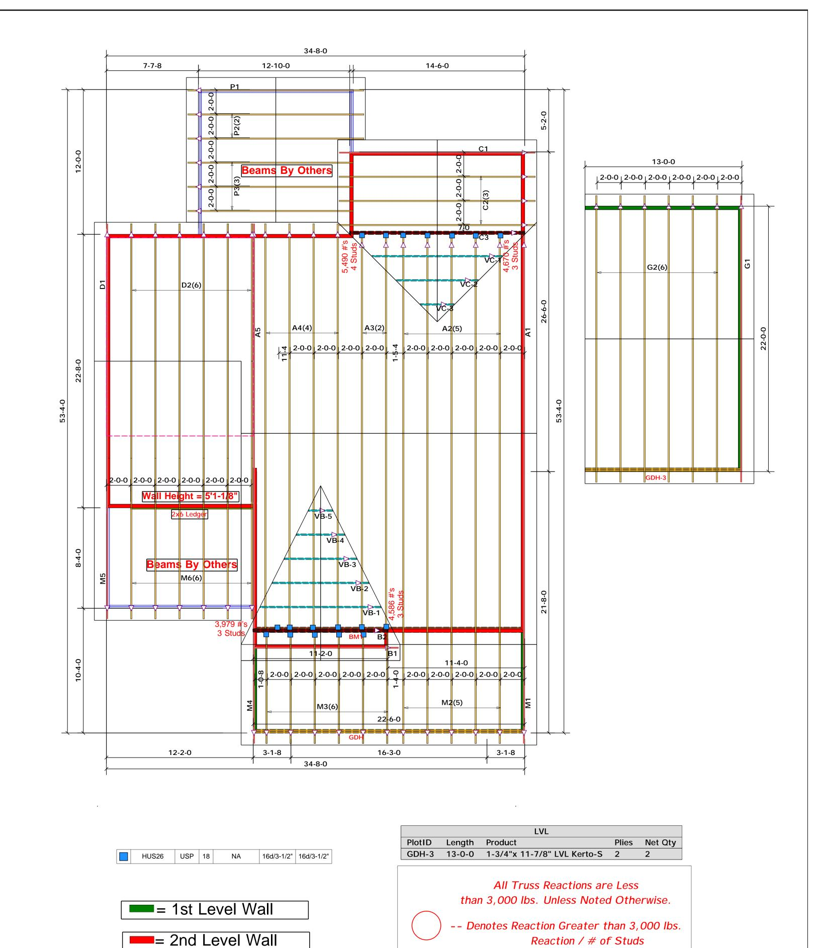
**Truss Placement Plan** SCALE: 1/4"=1'
