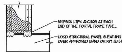
OVER RAISED WOOD FLOOR - FRAMING ANCHOR OPTION * APPLICABLE W/ GREATER THAN 12" KNEE WALL HEIGHTS IN CRAWL SPACE AND ABOVE FRAMED BASEMENT WALLS *
