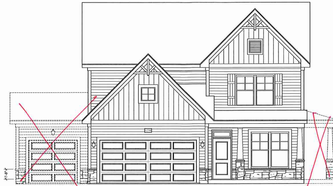
FRONT ELEVATION-B-2 (W/ STONE) SCALE: 1/4" = 1'-0"
