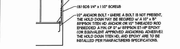
HOLD DOWN DETAIL FOR MASONRY FOUNDATION OR MONOLITHIC SLAB ④ * APPLICABLE ONLY WHERE SPECIFIED ON PLAN *
