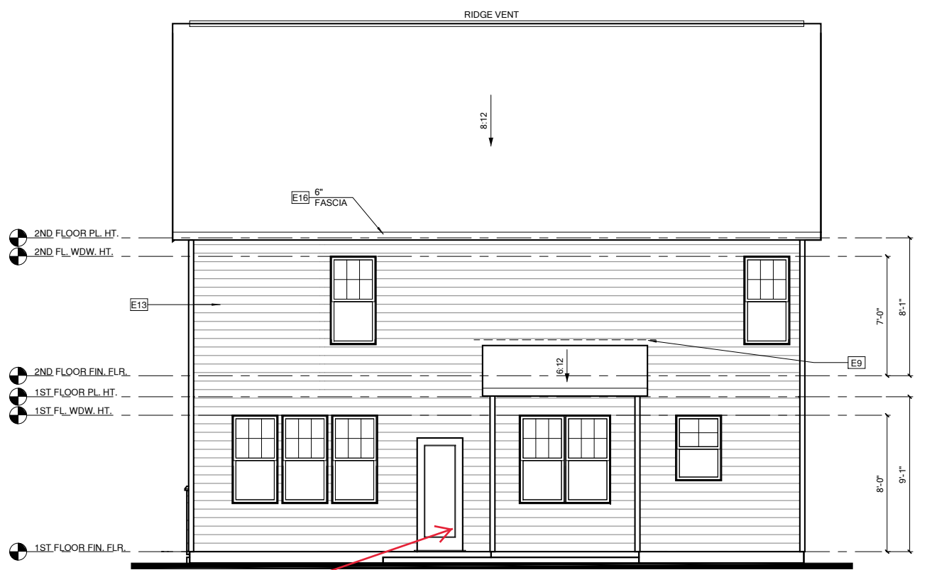
REAR ELEVATION 'CRAFTSMAN' CRAWL FOUNDATION
