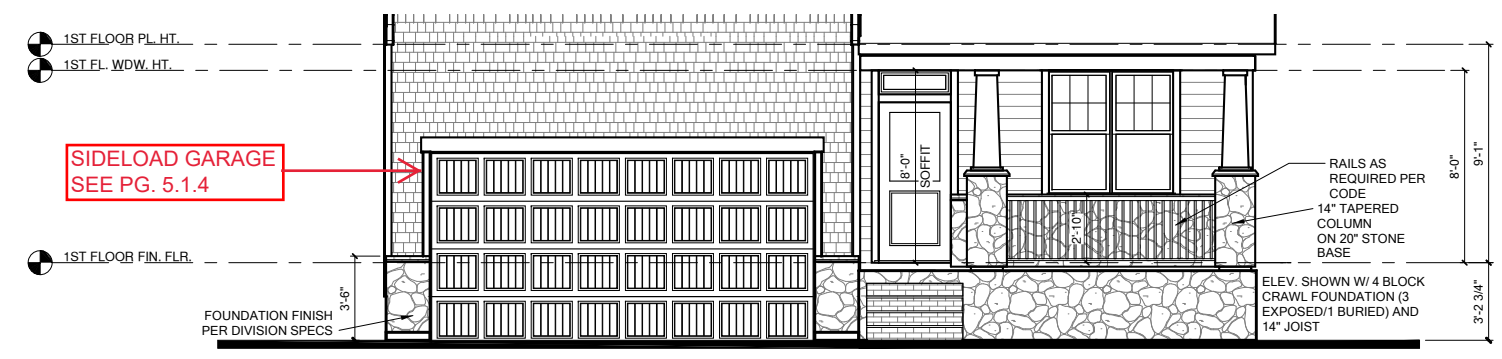
FRONT ELEVATION 'CRAFTSMAN' W/ CRAWL SPACE 1/4" = 1'-0" AT 22"X34" LAYOUT 1/8" = 1'-0" AT 11" X 17" LAYOUT
