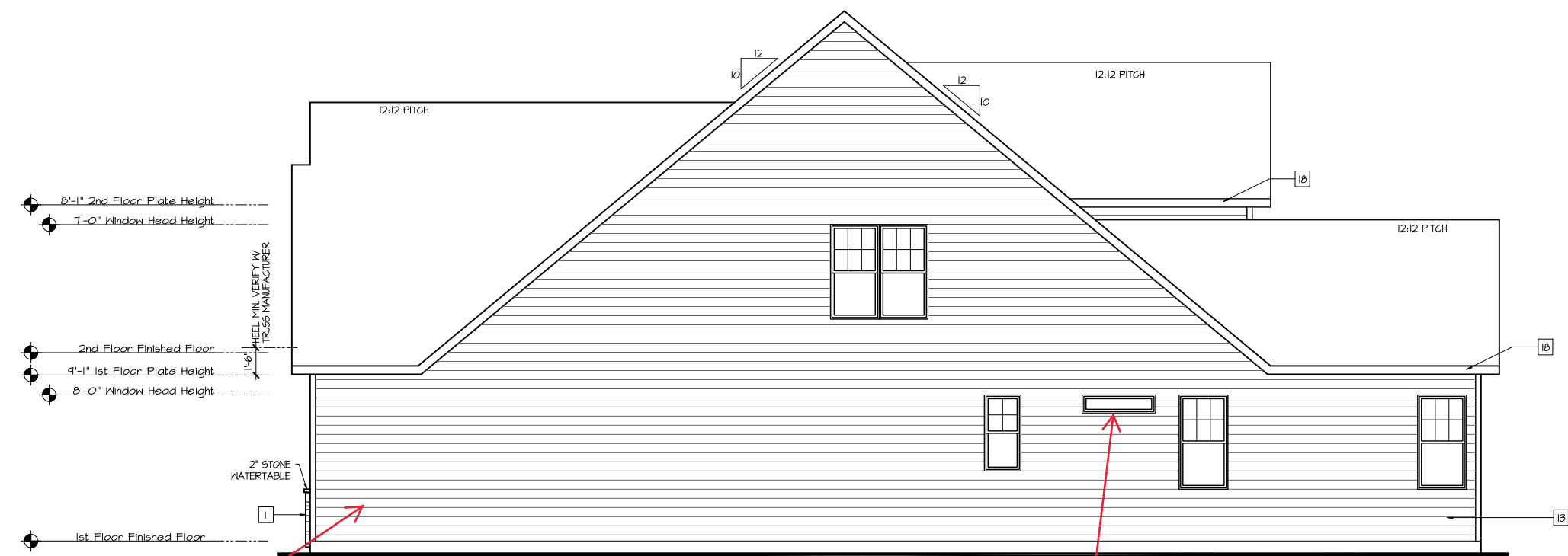
Right Elevation 'Craftsman' W/ Opt Loft SCALE: 1/4"=1'-0" AT 22"X34" LAYOUT 1/8"=1'-0" AT 11"X17" LAYOUT
