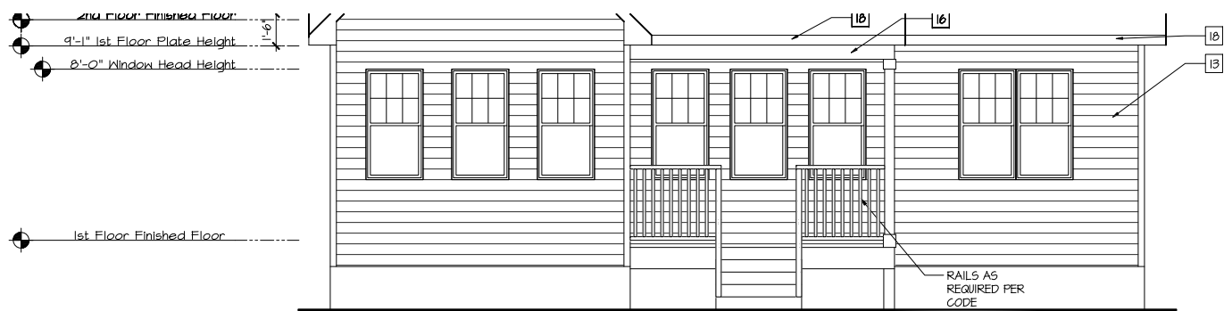
Rear Elevation 'Craftsman' w/ Crawlspace
