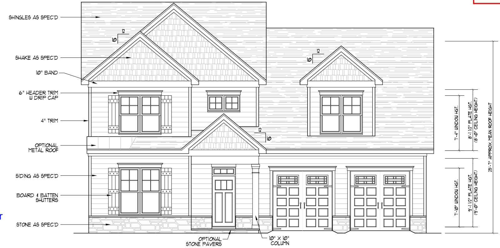
THIS PLAN CONFORMS TO THE 2018 EDITION OF THE I.R.C. / NORTH CAROLINA RESIDENTIAL CODE. FRONT ELEVATION "A" SCALE: ----- 1/8" = 1'-0" STONE OPTION #1
