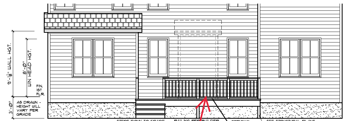
REAR ELEVATION w/ CRAWL FND. WOOD DECKING 22x34 PRINTS SCALE: 1/4"=1'-0" 11x17 PRINTS SCALE: 1/8"=1'-0"
