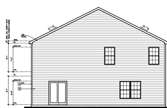
Rear Elevation 'C' SCALE: 1/8"=1'-0" AT 22"x34" LAYOUT 1/8"=1'-0" AT 11"x11" LAYOUT
