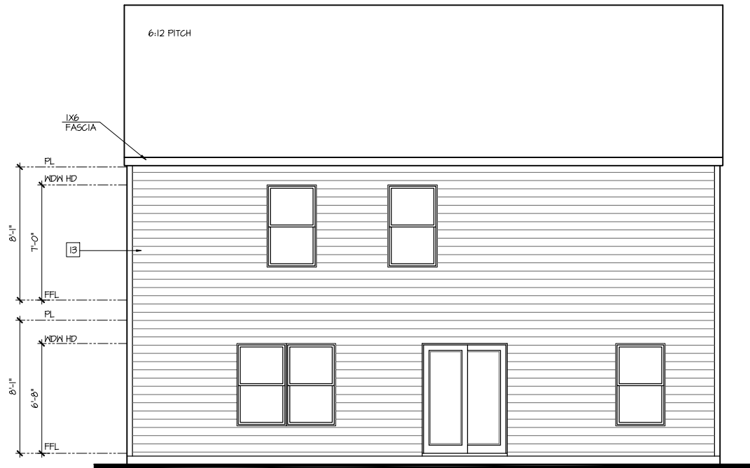
Rear Elevation 'K' SCALE: 1/4"=1'-0" AT 22'X34' LAYOUT 1/8"=1'-0" AT 11'X11" LAYOUT
