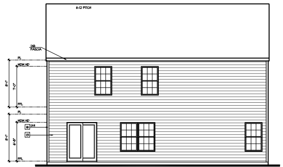
Rear Elevation 'C' SCALE: 1/4"=1'-0" AT 22'X34' LAYOUT 1/8"=1'-0" AT 11'X11' LAYOUT
