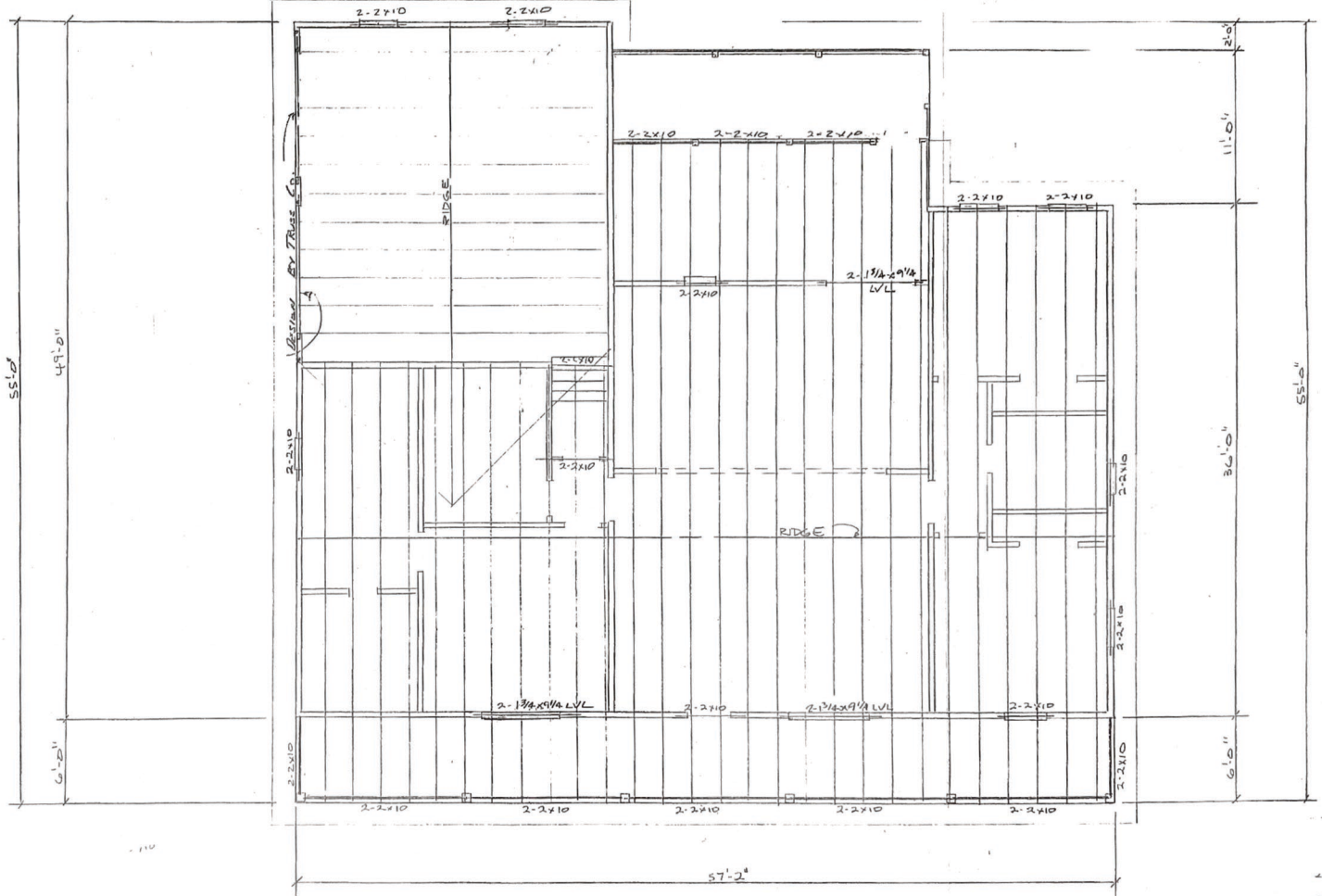
ROOF FRAMING PLAN SCALE 1/8" = 1'-0"
