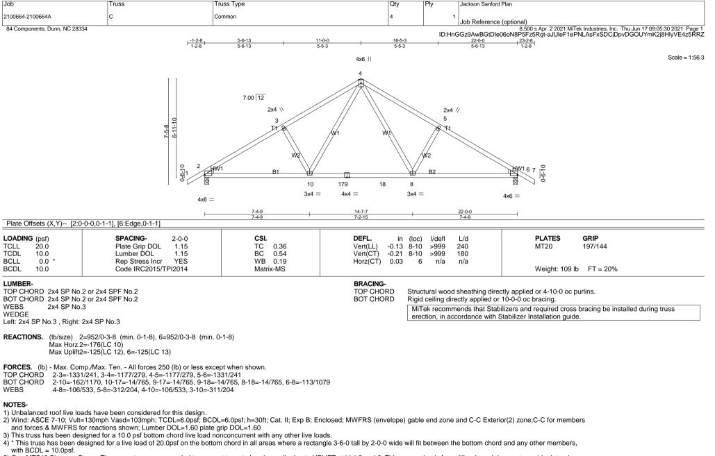
5) One MTS12 Simpson Strong-Tie connectors recommended to connect truss to bearing walls due to UPLIFT at jt(s) 2 and 6. This connection is for uplift only and does not consider lateral forces.
