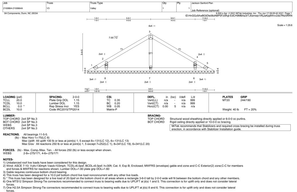
8) This truss is designed in accordance with the 2015 International Residential Code sections R502.11.1 and R802.10.2 and referenced standard ANSI/TPI 1.
