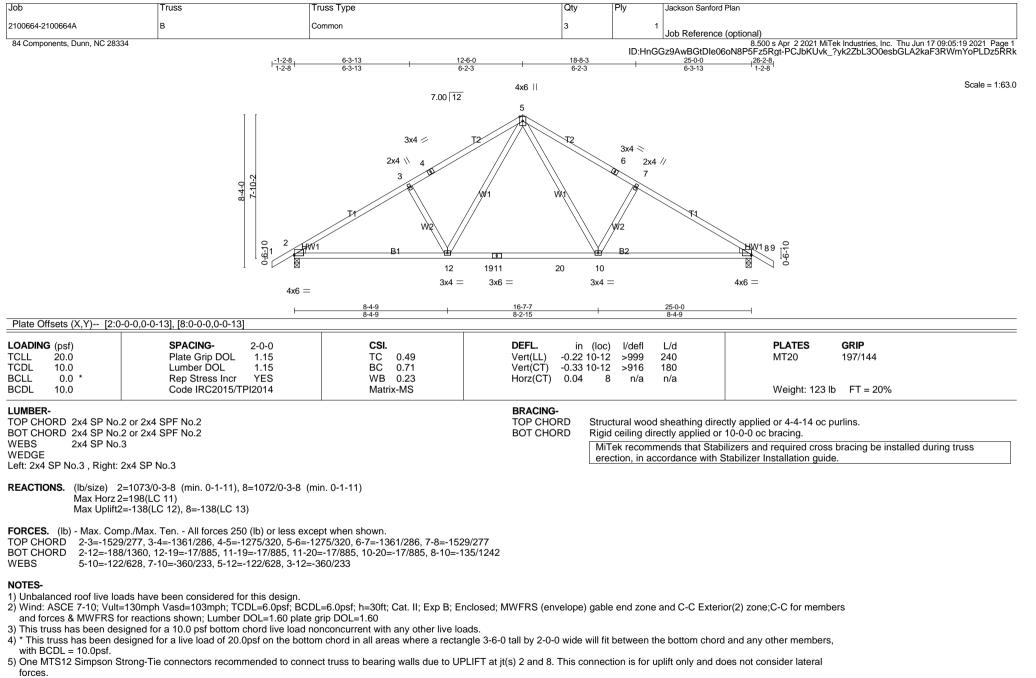
6) This truss is designed in accordance with the 2015 International Residential Code sections R502.11.1 and R802.10.2 and referenced standard ANSI/TPI 1.
