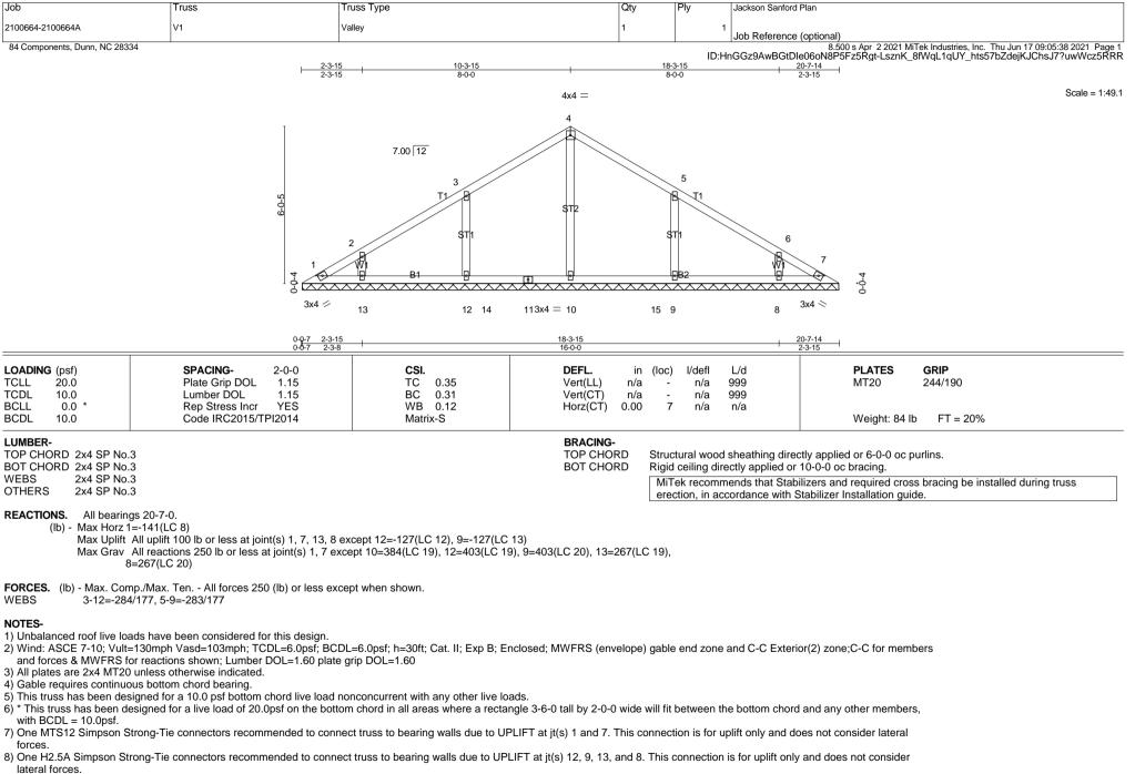
9) This truss is designed in accordance with the 2015 International Residential Code sections R502.11.1 and R802.10.2 and referenced standard ANSI/TPI 1.
