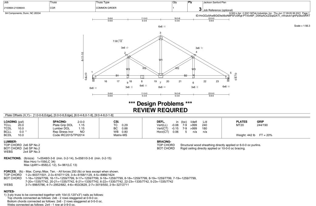
2) All loads are considered equally applied to all plies, except if noted as front (F) or back (B) face in the LOAD CASE(S) section. Ply to ply connections have been provided to distribute only loads noted as (F) or (B), unless otherwise indicated.
