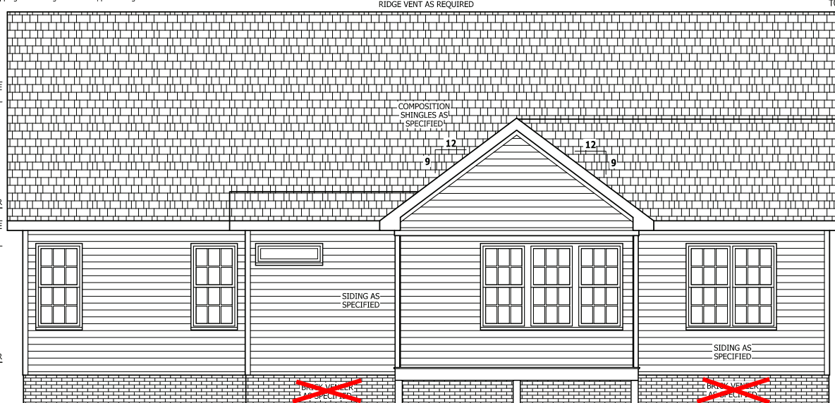
REAR ELEVATION SCALE 1/4" = 1'-0"
