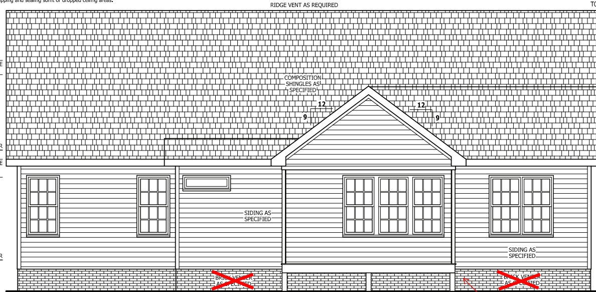
REAR ELEVATION SCALE 1/4" = 1'-0"
