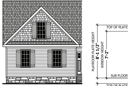
GARAGE FRONT WITH OPTIONAL SIDE LOAD SCALE 1/8" = 1'-0"
