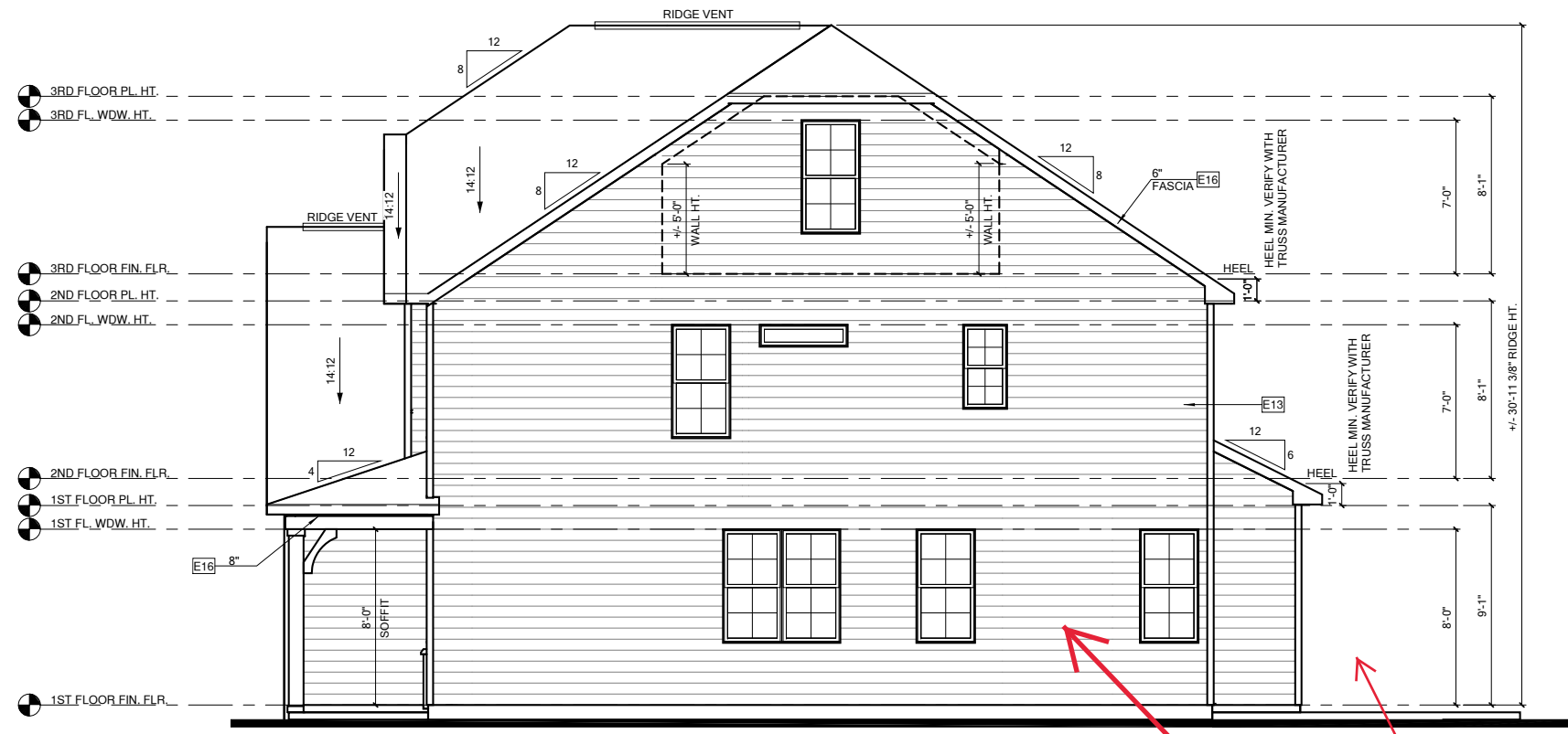
RIGHT ELEVATION 'EURO' CRAWL FOUNDATION 1/4" = 1'-0" AT 22"X34" LAYOUT 1/8" = 1'-0" AT 11" X 17" LAYOUT FIREPLACE SEE PG. 5.1.3 COVERED DECK SEE PG. 5.1.2
