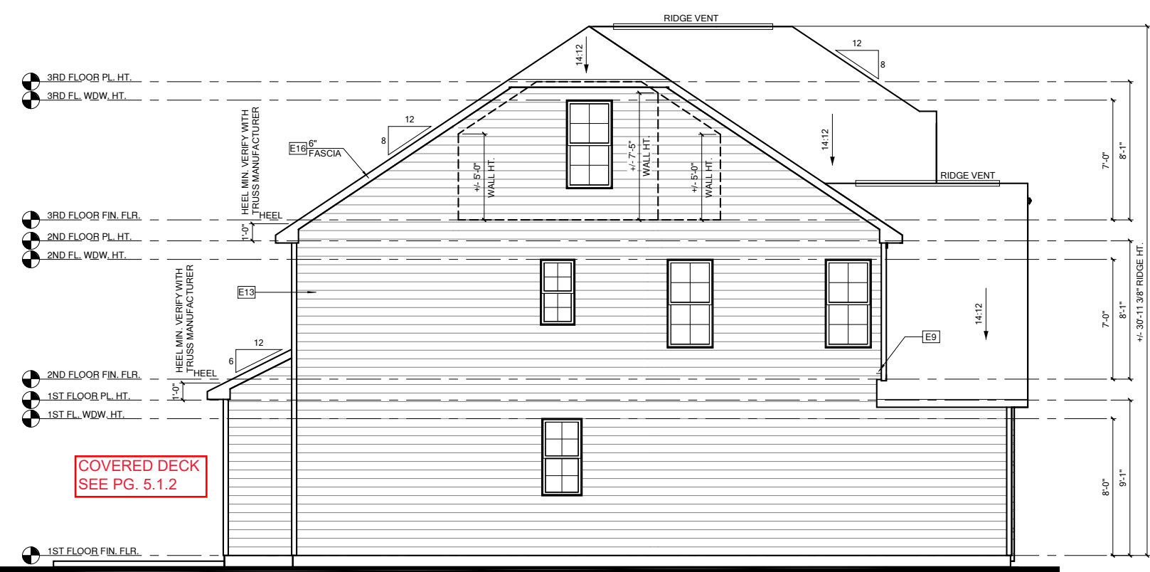
LEFT ELEVATION 'EURO' 1/4" = 1'-0" AT 22"X34" LAYOUT 1/8" = 1'-0" AT 11" X 17" LAYOUT COVERED DECK SEE PG. 5.1.2 CRAWL FOUNDATION
