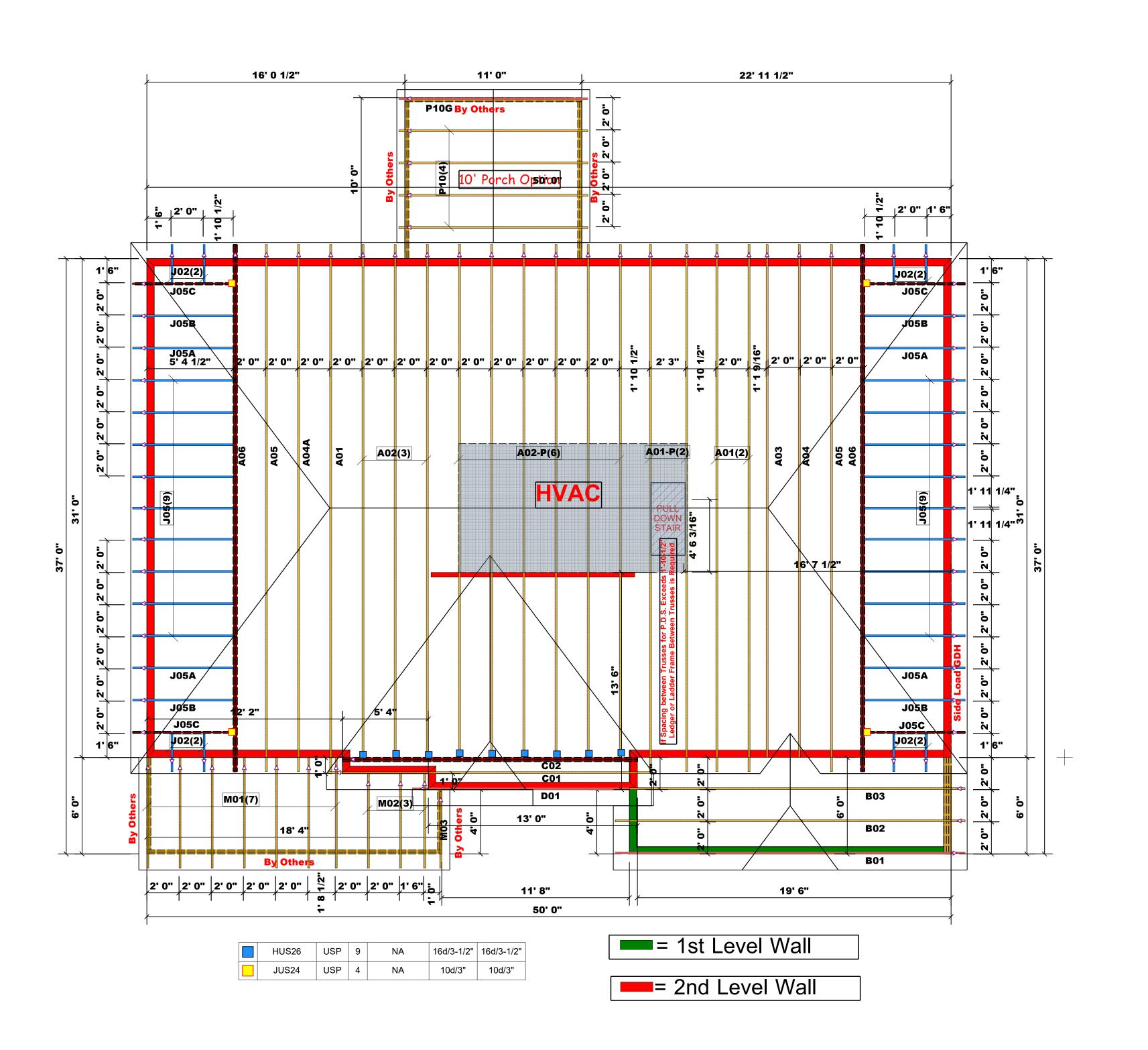
ROOF & FLOOR TRUSSES & BEAMS
