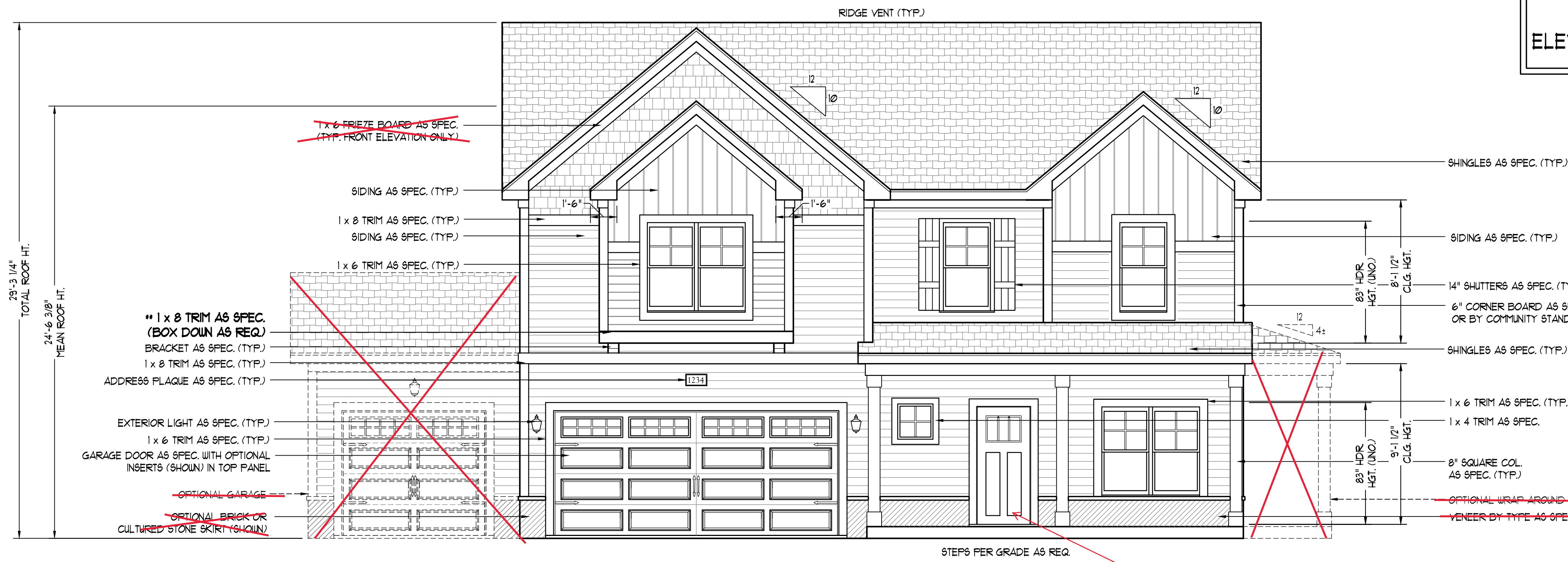
FRONT ELEVATION-B SCALE: 1/4" = 1'-0"
