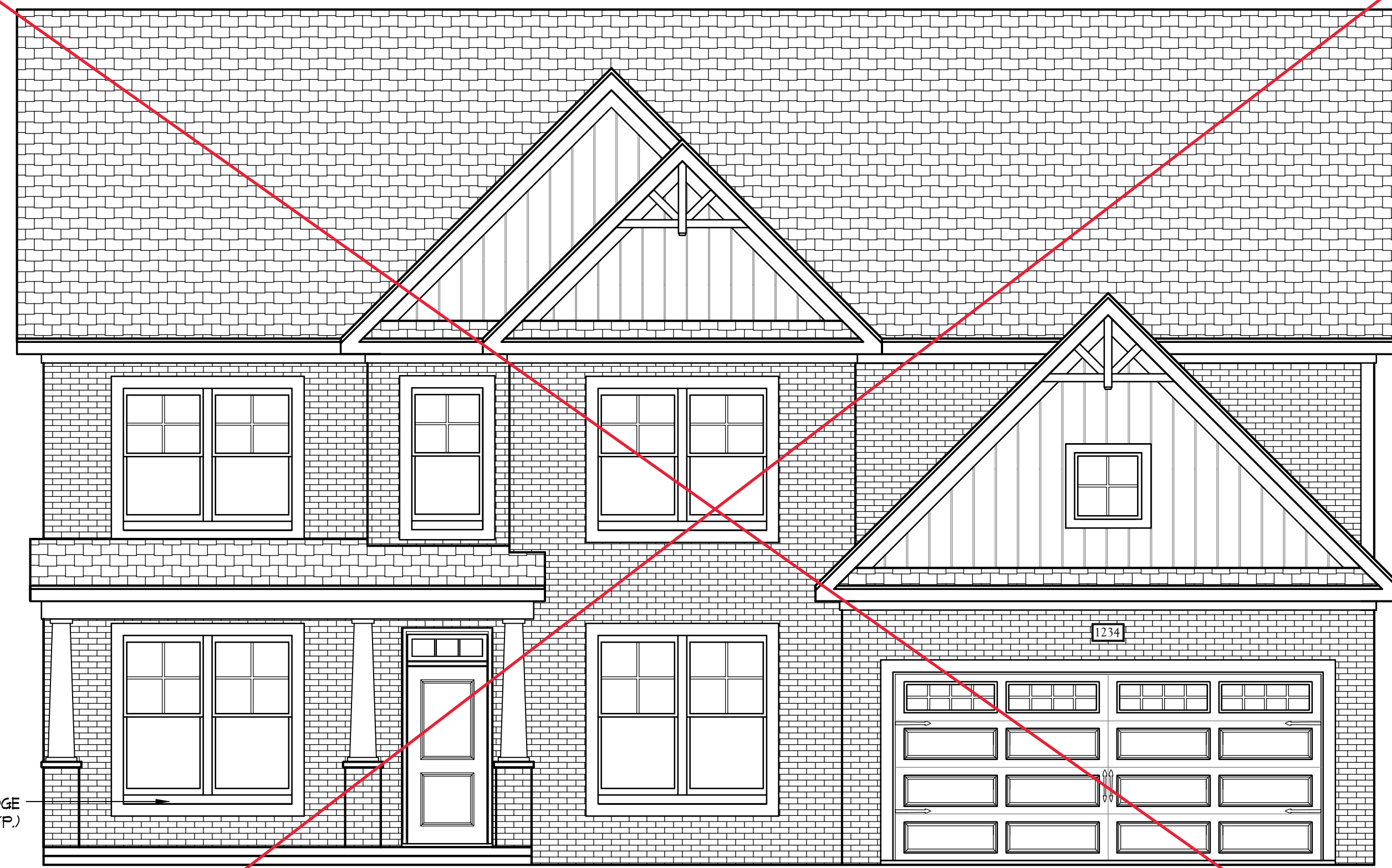
FRONT ELEVATION-B-4 SCALE: 1/4" = 1'-0"
