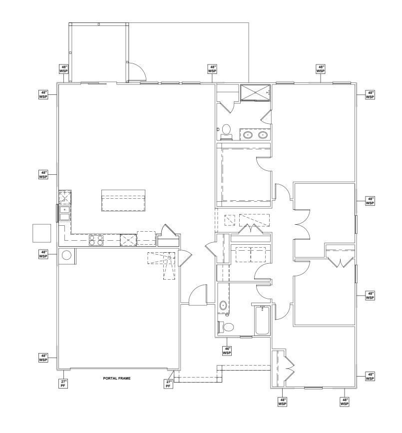
FIRST FLOOR WALL BRACING PLAN - 'C'
