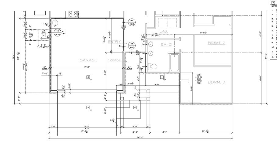
PARTIAL SLAB INTERFACE PLAN 'C'
