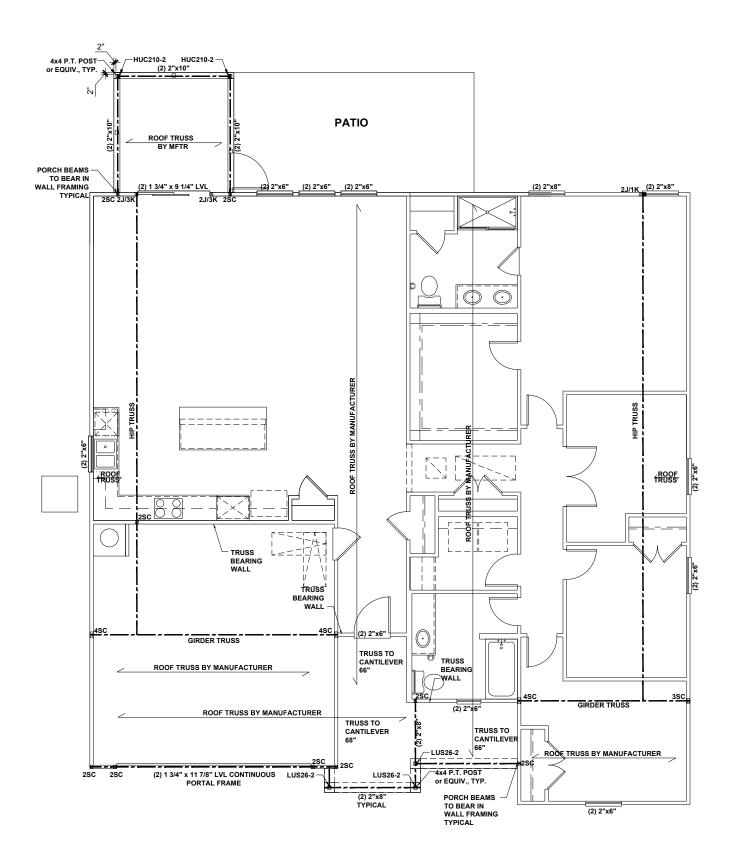
FIRST FLOOR CEILING FRAMING PLAN - 'C'
