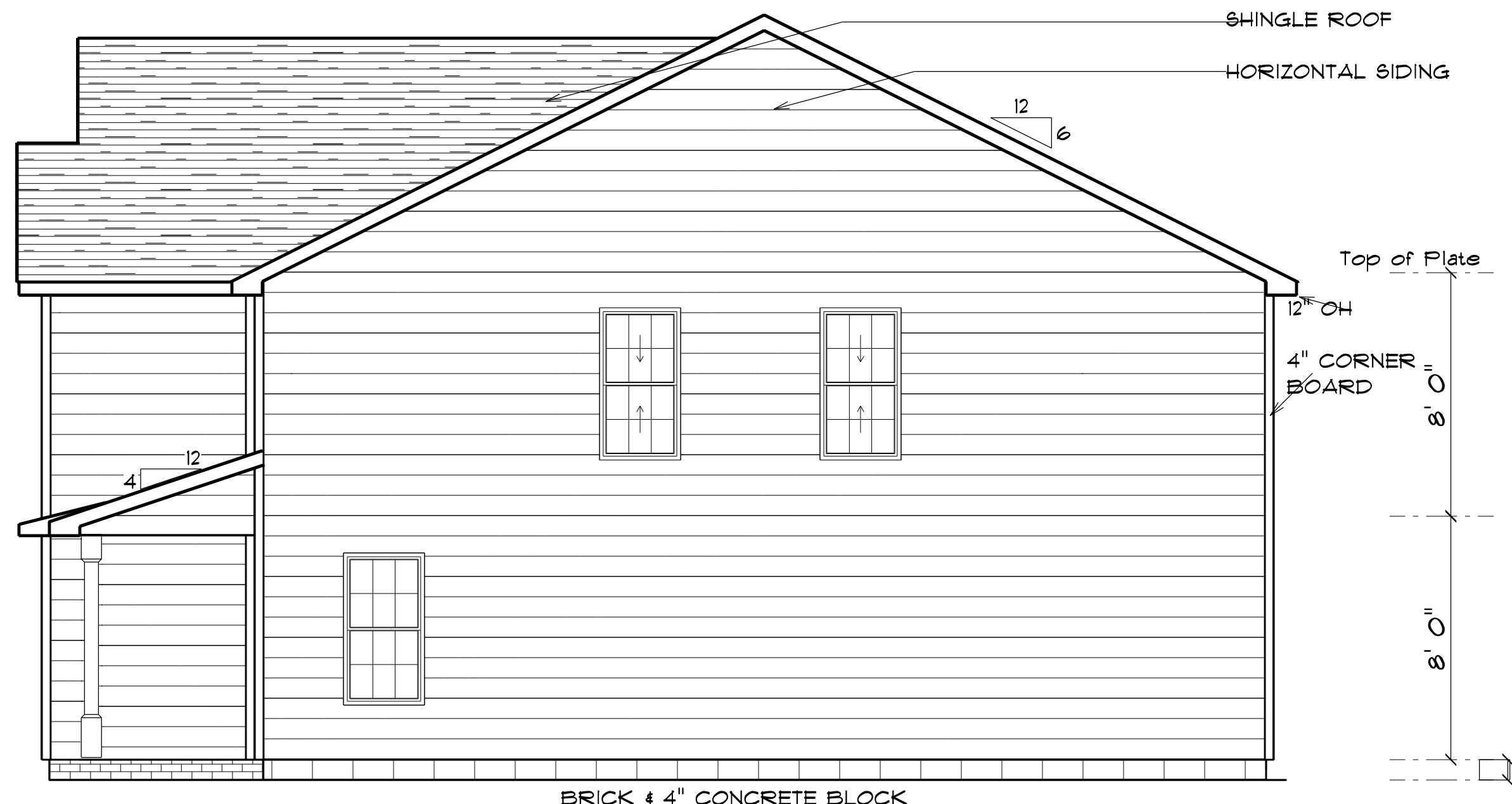
LEFT ELEVATION SCALE: 1" = 1/4"
