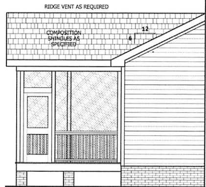
LEFT SIDE ELEVATION SCALE 1/4" = 1'-0"
