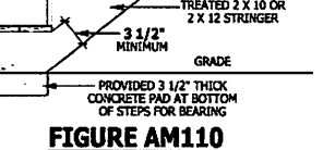
H TYPICAL DECK STAIR DETAIL SCALE 3/4" = 1'-0"
