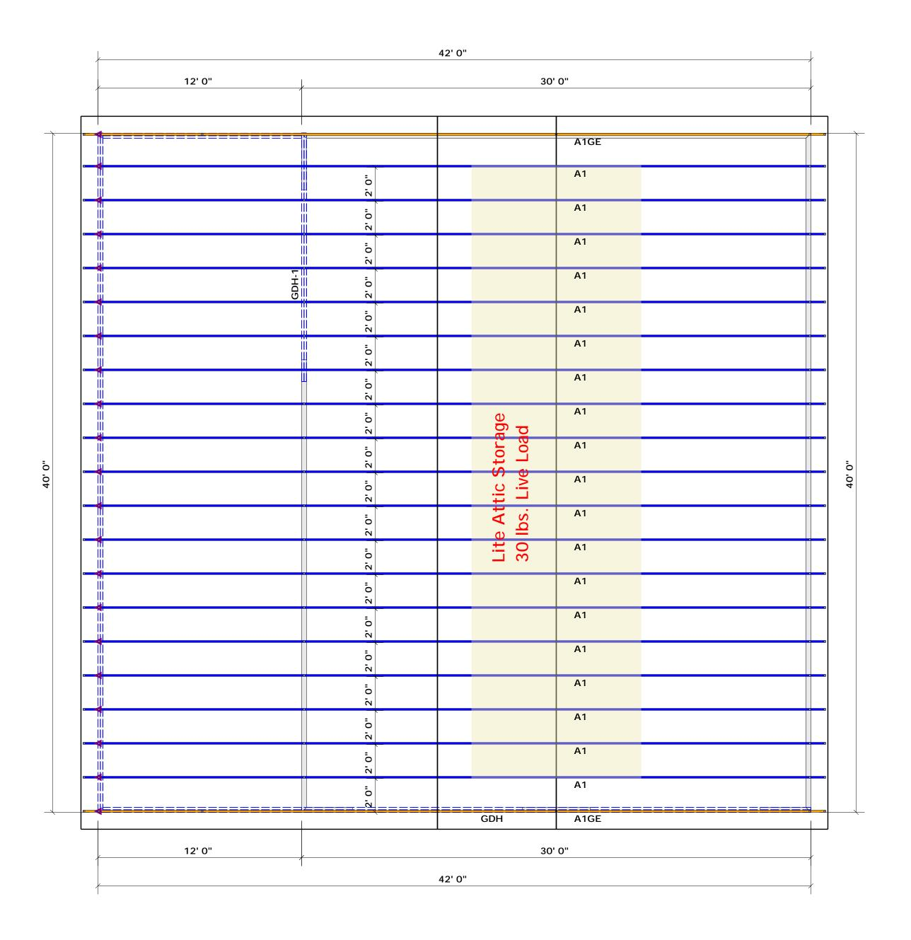
Truss Placement Plan
