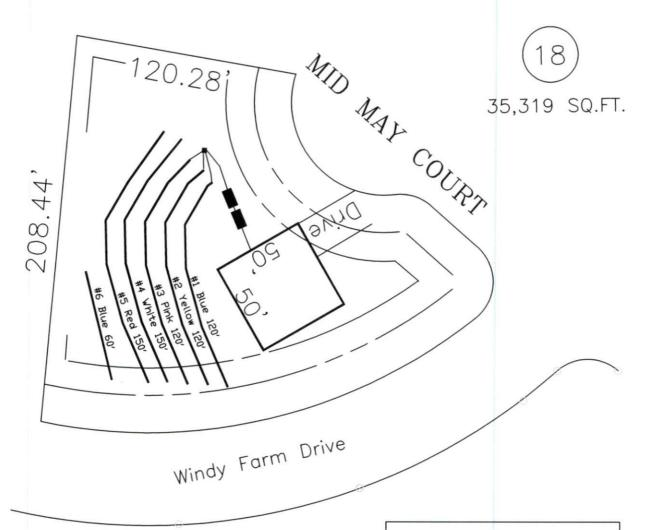
System: Pump to D-Box Lines: 1-3 (360') 0.35 LTAR 24" Trench Bottom Accepted Status System Repair: Pressure Manifold Lines: 4-6 (360') 0.35 LTAR 24 Trench Bottom Accepted Status System This drawing represents a preliminary septic plan made prior to final construction activities. A revised plan may need to be reworked at time of permitting.
