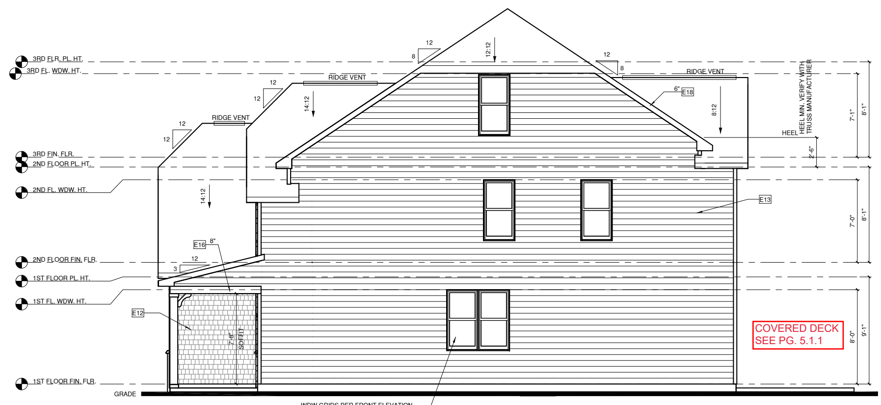
RIGHT ELEVATION EURO 1/4" = 1'-0" AT 22"X34" LAYOUT 1/8" = 1'-0" AT 11" X 17" LAYOUT FOUNDATION BRICK WRAP (3 SIDES)
