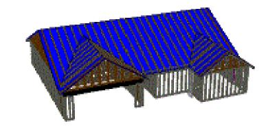
THE PURPOSE OF THIS DETAIL IS TO ILLUSTRATE HOW TO PROPERLY SPACE 24" O.C. ROOF TRUSSES TO ALLOW FOR A 25 1/2" OPENING FOR PULL DOWN ATTIC ACCESS
