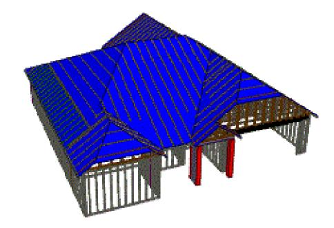
THE PURPOSE OF THIS DETAIL IS TO ILLUSTRATE HOW TO PROPERLY SPACE 24" O.C. ROOF TRUSSES TO ALLOW FOR A 25 1/2" OPENING FOR PULL DOWN ATTIC ACCESS
