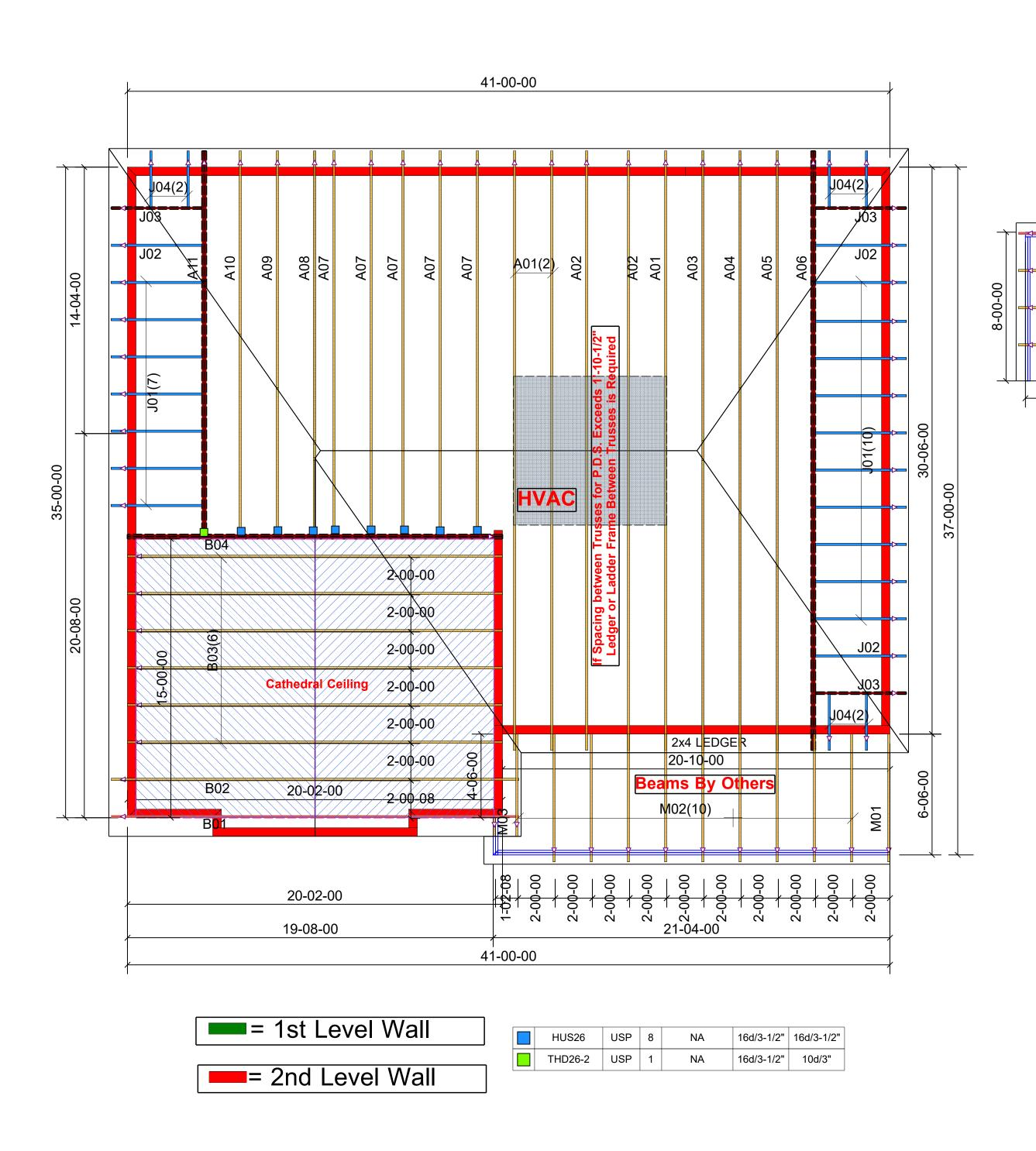
ROOF & FLOOR TRUSSES & BEAMS
