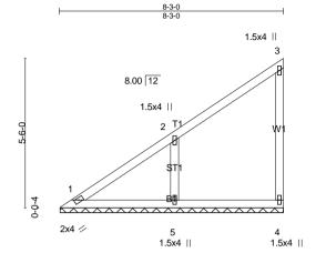
LOADING (psf) SPACING-2-0-0 CSI. TC Plate Grip DOL TCLL 20.0 1.15 0.41 0.25 **TCDL** 10.0 Lumber DOL 1.15 BC WB 0.07 **BCLL** 0.0 \* Rep Stress Incr YES BCDL 10.0 Code IRC2015/TPI2014 Matrix-P
