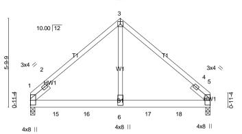
11-8-0 5-10-0 LOADING (psf) SPACING-2-0-0 CSI. DEFL. in (loc) I/defl TCLL 20.0 Plate Grip DOL 1.15 TC 0.47 Vert(LL) 0.05 6-13 >999 **TCDL** 10.0 Lumber DOL 1.15 BC 0.63 Vert(CT) -0.06 6-13 >999 **BCLL** 0.0 \* Rep Stress Incr NO WB 0.41 Horz(CT) 0.02 n/a BCDL 10.0 Code IRC2015/TPI2014 Matrix-MS
