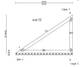
CSI. LOADING (psf) SPACING-2-0-0 TC 0.89 TCLL 20.0 Plate Grip DOL 1.15 ВС 0.56 TCDL 10.0 Lumber DOL 1.15 WB 0.00 **BCLL** 0.0 \* Rep Stress Incr YES
