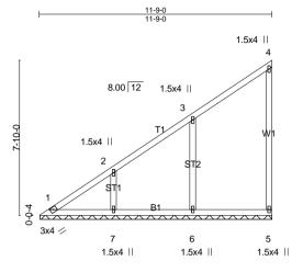
**PLATES** LOADING (psf) SPACING-2-0-0 CSI. DEFL. in (loc) I/defl L/d **GRIP** TC 0.19 TCLL 20.0 Plate Grip DOL 1.15 Vert(LL) n/a n/a 999 MT20 197/144 0.29 **TCDL** 10.0 Lumber DOL 1.15 BC Vert(CT) n/a 999 n/a WB 0.13 **BCLL** 0.0 \* Rep Stress Incr YES Horz(CT) 0.00 5 n/a n/a BCDL 10.0 Code IRC2015/TPI2014 Matrix-S Weight: 58 lb FT = 20%
