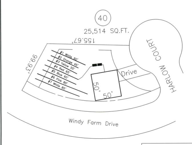
This drawing represents a preliminary septic plan made prior to final construction activities. A revised plan may need to be reworked at time of permitting.
