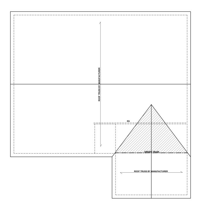
**ROOF FRAMING PLAN - 'A'**
