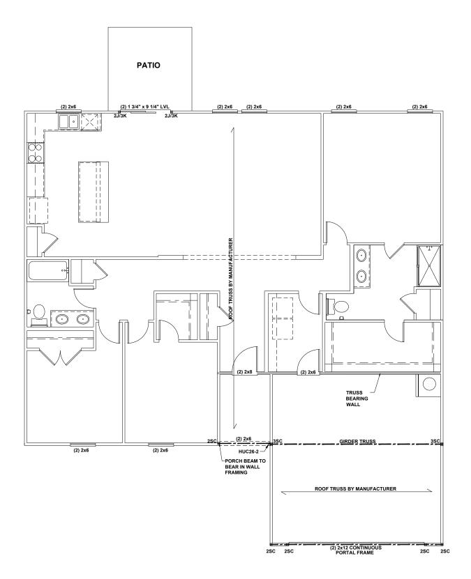
**FIRST FLOOR CEILING FRAMING PLAN - 'A'**
