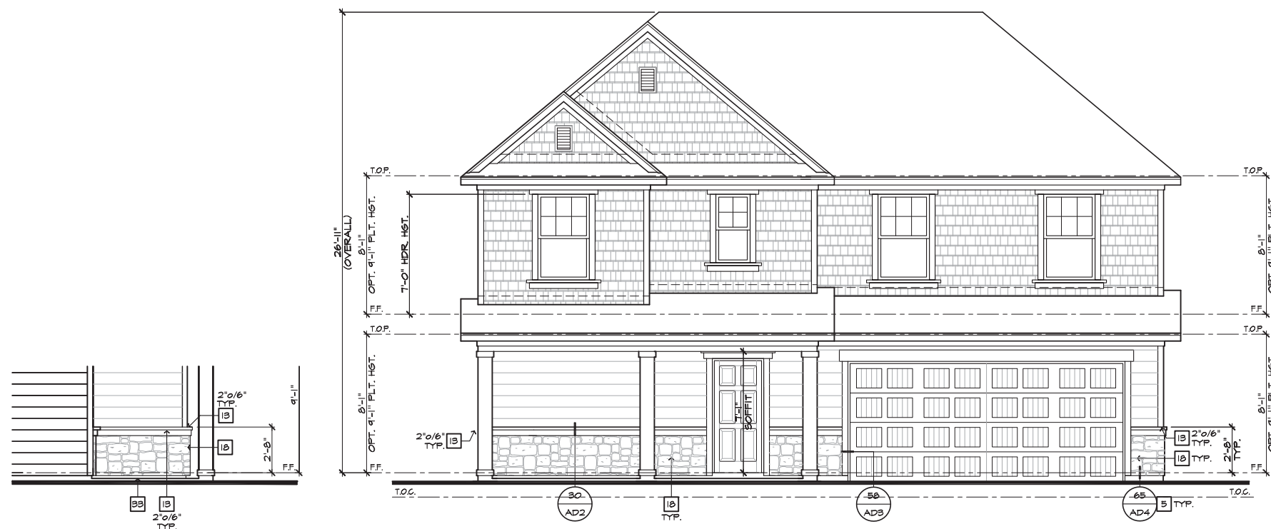
LEFT ELEVATION 'D' W/ OPTIONAL STONE AT OPTIONAL 9'-1" PLT. HGT. SCALE 1/4"=1'-0" (22"X34") - 1/8"=1'-0" (11"X17")
